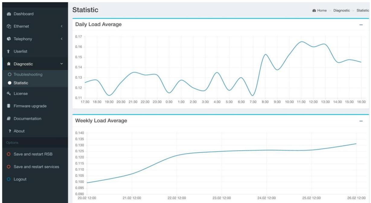
The graph «Daily Load Average» features timely averaged scheme of processor load for the latter 24 hours. The system value «load average 15» is taken by default.
